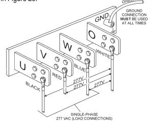
Figure 29. UVWO Terminal Lugs 1Ø-277V Connections
